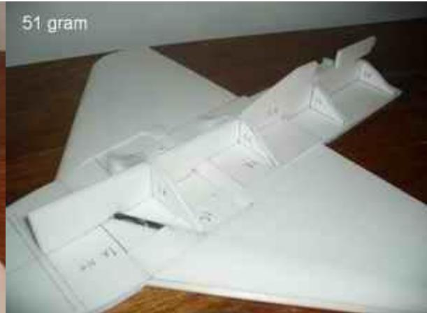
Cut and glue pieces 3A, B, C and D. Bevel 3A so it is flush with the formers, and can be sheeted later.
