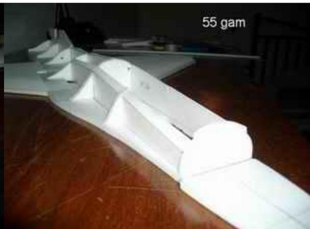
Install push rod outer tubes. Cut them flush with bottom so frame can still be built on a flat surface. They do have to exit with a pretty shallow angle on the bottom so they approach the horns on the right angle. Test with inner tubes, should run very free.
