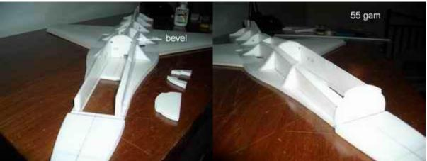
Install push rod outer tubes. Cut them flush with bottom so frame can still be built on a flat surface. They do have to exit with a pretty shallow angle on the bottom so they approach the horns on the right angle. Test with inner tubes, should run very free.
