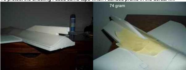
The top is now finished. This is a good time to score some panel lines on the top because it is still flat on the table. To score I use the dull side of a tableknife. Use a piece of tape where you want the panel line and follow it with the knife. No need to press very hard, you only want to dent it, not partly cut it. My lines are semi-scale. Use the topview to determine where a line should be. It will look great even if not all lines are there or in the right place.
