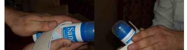
Cut the LH and RH cockpit sheeting. Preform it with a spraycan and your fingers. Glue the top first. When that is cured put glue on the formers and bottom plate. Spray some accelerator in there and fold it down. Hold with your hands untill cured.
