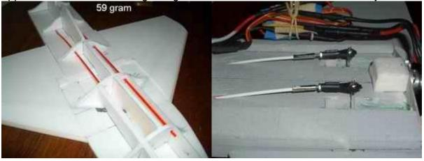
Cut 4 pieces of 4A and some 6X6 mm depron pieces. Glue in place in tail section.
