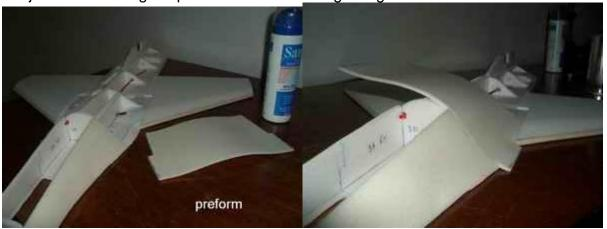
If you have beveled the bottom plate enough before, the wing / fuselage joint will be nice and smooth.
