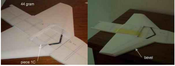
Glue 4 mm wide balsastrips to the leading edge and sand to shape. Cut and glue piece 2A to frame using the penlines drawn before.
