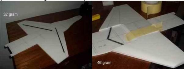
Cut out and slot two pieces 1C (3 mm depron 30 X 100 mm) so they can be glued on the CF spars.
