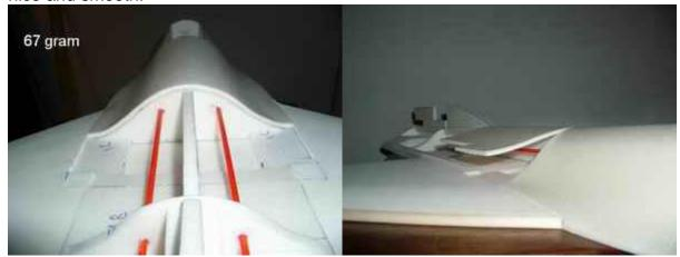
Cut the aft middle sheeting. Preform and trial fit. Check the blue line to see what you try to achieve. After the thickest point in the wing the aft fuselage is perpendicular to the wing, this was also already achieved during the wingprofile sanding process and now you add 3 mm sheeting to it
